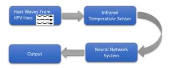
FIGURE 1: Main structure of the proposed heat wave measuring system.
