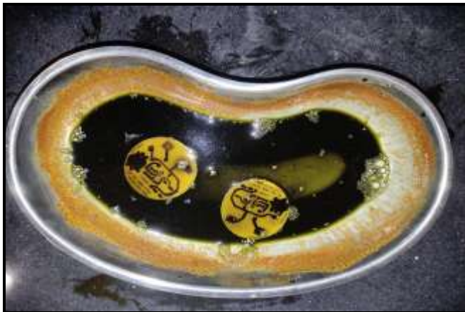
FIGURE 6. Preparation of circuit on copper board
