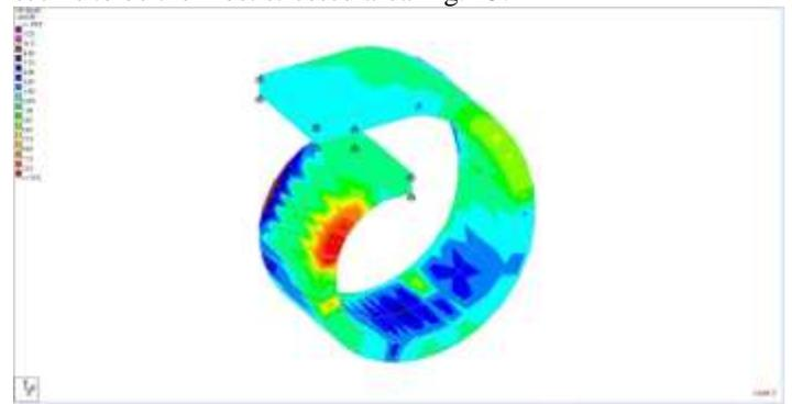
FIGURE 15. Maximum Flexural Stress Diagram
