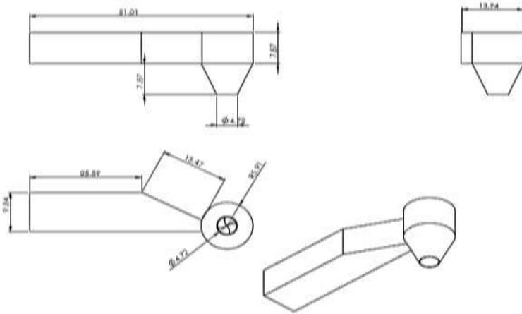
FIGURE 2. GWVTPP Turbine Design all dimensions in cm
