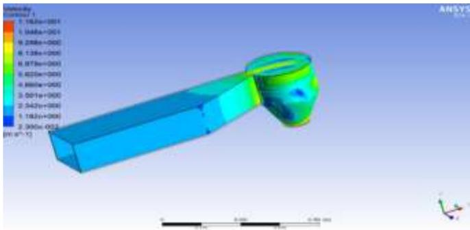
FIGURE 10. Wall velocity contour of inlet channel having notch angle of 153
