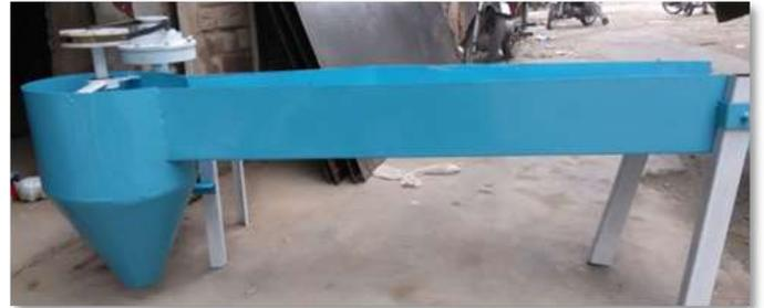
FIGURE 6. Gravitational Vortex Turbines Side View
