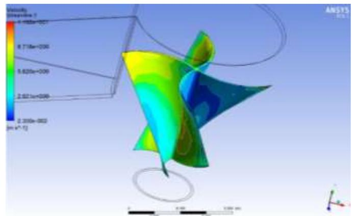
FIGURE 9. Velocity stream lines and the distribution from center to edges
