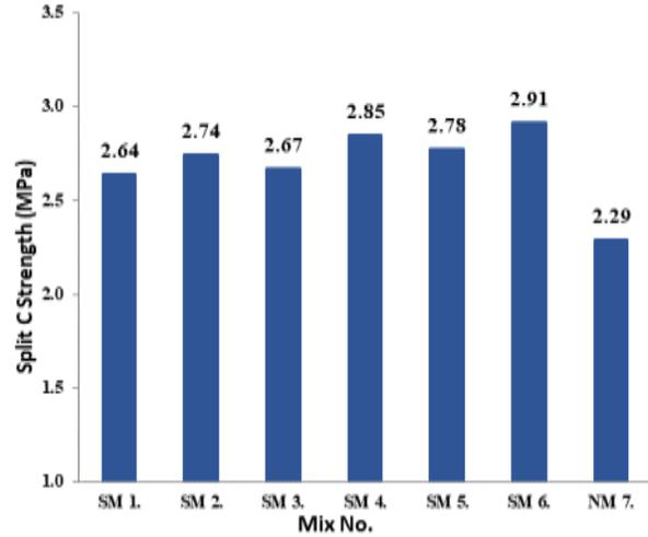
b) split tensile strength Test
