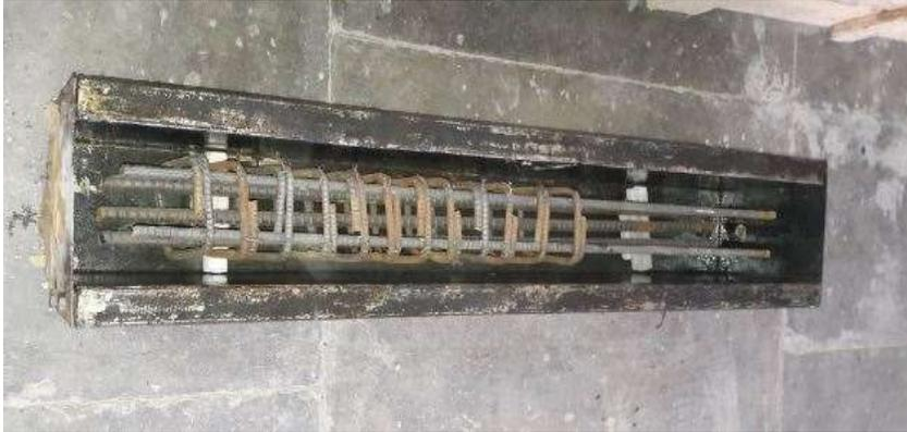
a) Steel Reinforcement Cage
