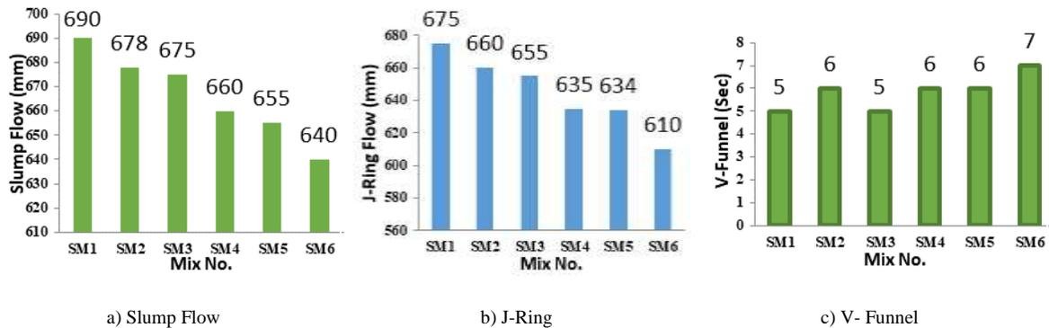
FIGURE 5: Fresh SCC Tests of Prepared Mixes
