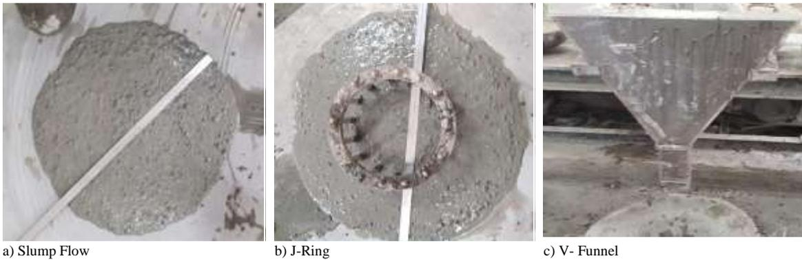
FIGURE 4: Fresh SCC Tests of Prepared Mixes
