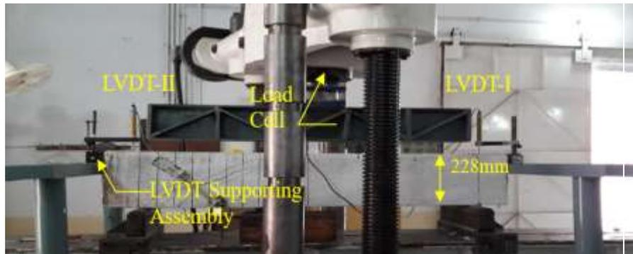
FIGURE 3: Test Setup for Shear Strength Test
