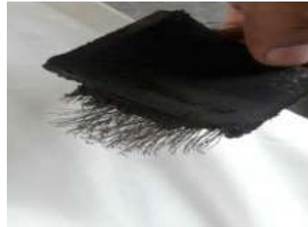
**d) Steel fibers in a waste tire piece**
