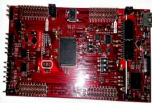
Figure 18: Launchpad Board To control the gate signal of bridges, a I-phase step up and down regulator was required as shown in the figure below. Thus the BOOSTXL-DRV8305EVM was utilized as a Dual Active Bridge (DAB) Converter.
