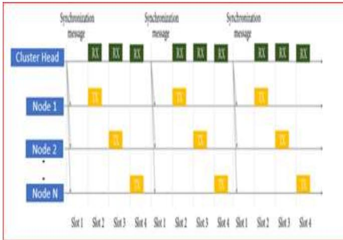
FIGURE 1: Time allocation for Time slot by the receiver node
