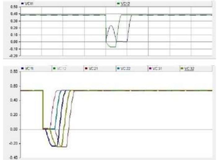
FIGURE 7. Commutation Capacitor Voltages
