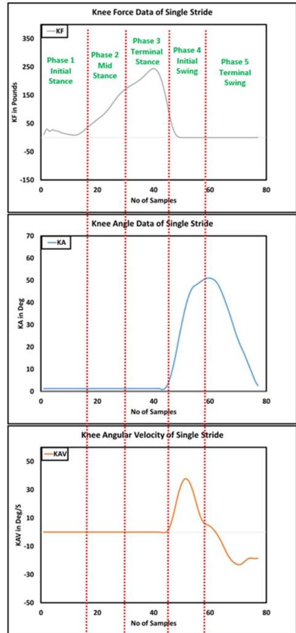
Figure 2. Semi-active prosthetic knee sensors data.
