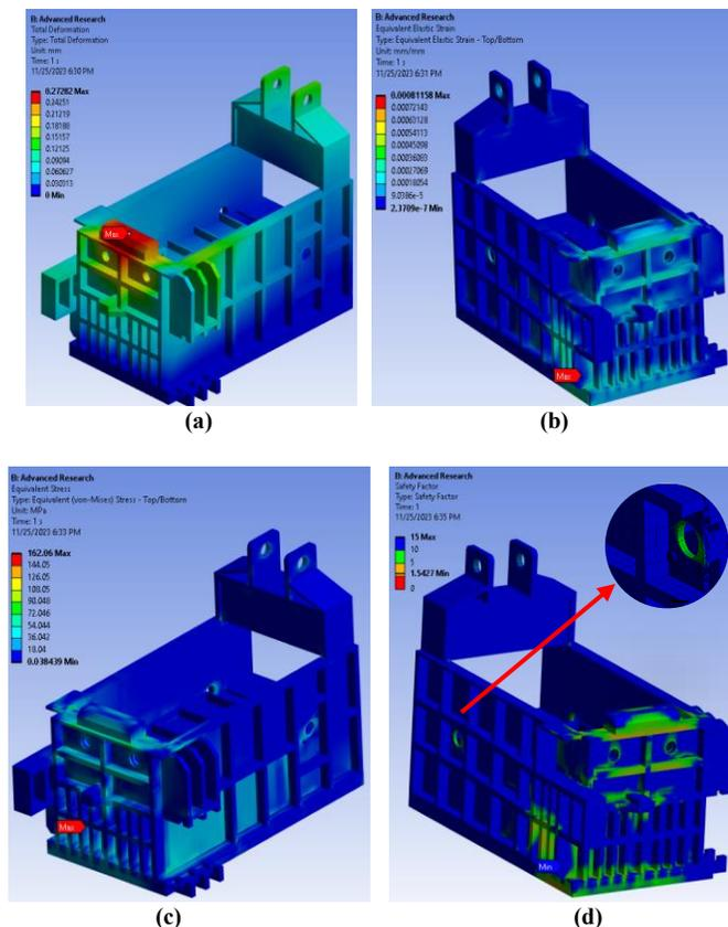
**Figure 11.** Bolt pretension analysis results (a) Maximum deformation; (b) Maximum Equivalent Strain; (c) Maximum Equivalent Stress; (d) Safety Factor.
