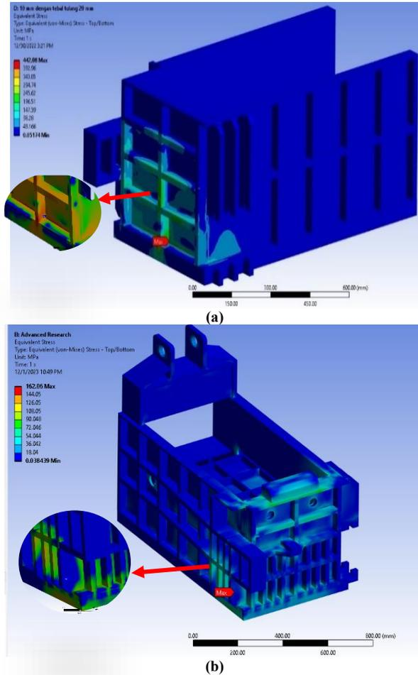
Figure 8. Design optimization (a) Design geometry 1,2, and 3 hydraulic press machines (b) Design geometry 4,5 with an increasing number of frames
