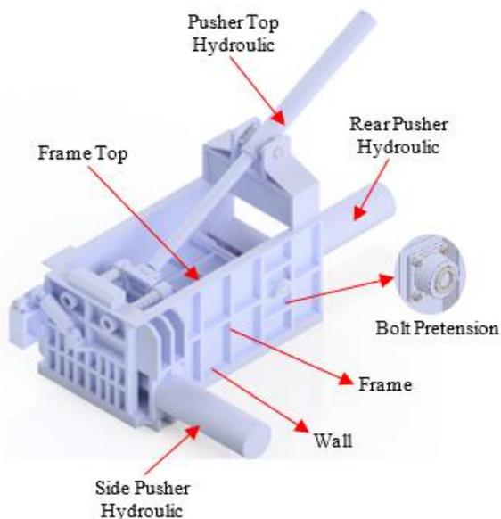
Figure 2. Hydraulic press machine components.
