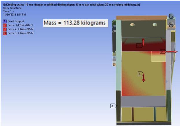
Figure 4. Boundary condition simulasi tahap 1 hydraulic press machine.
