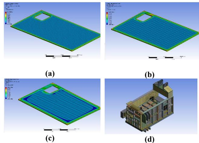
Figure 3. Mesh Convergence: (a) Element Size 45; (b) Element Size 35; (c) Element Size 25; (d) Mesh Geometry Machine.
