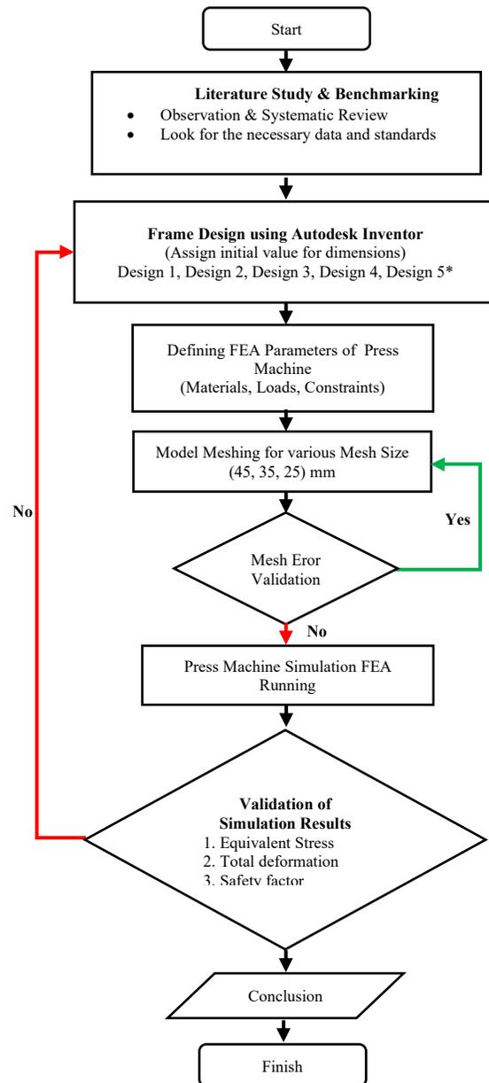
Figure 1. Workflow on design optimization press machine.
