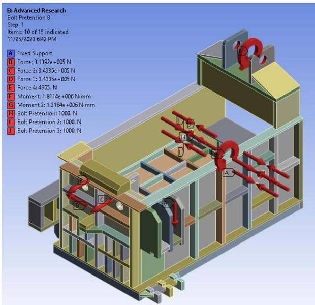
Figure 5. Loading limits of stage 2 hydraulic press machine simulation.
