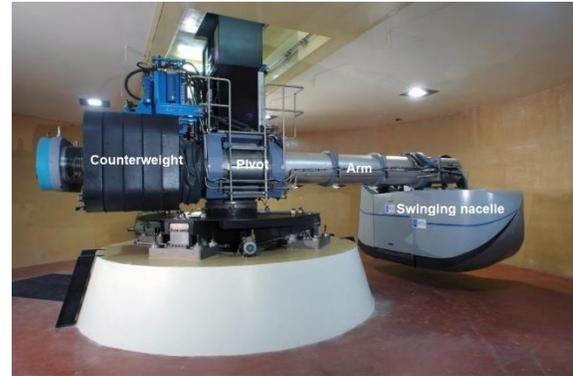
Figure 2. Scheme of centrifuge acceleration (Left) and photo of the IFSTTAR's centrifuge (right).
