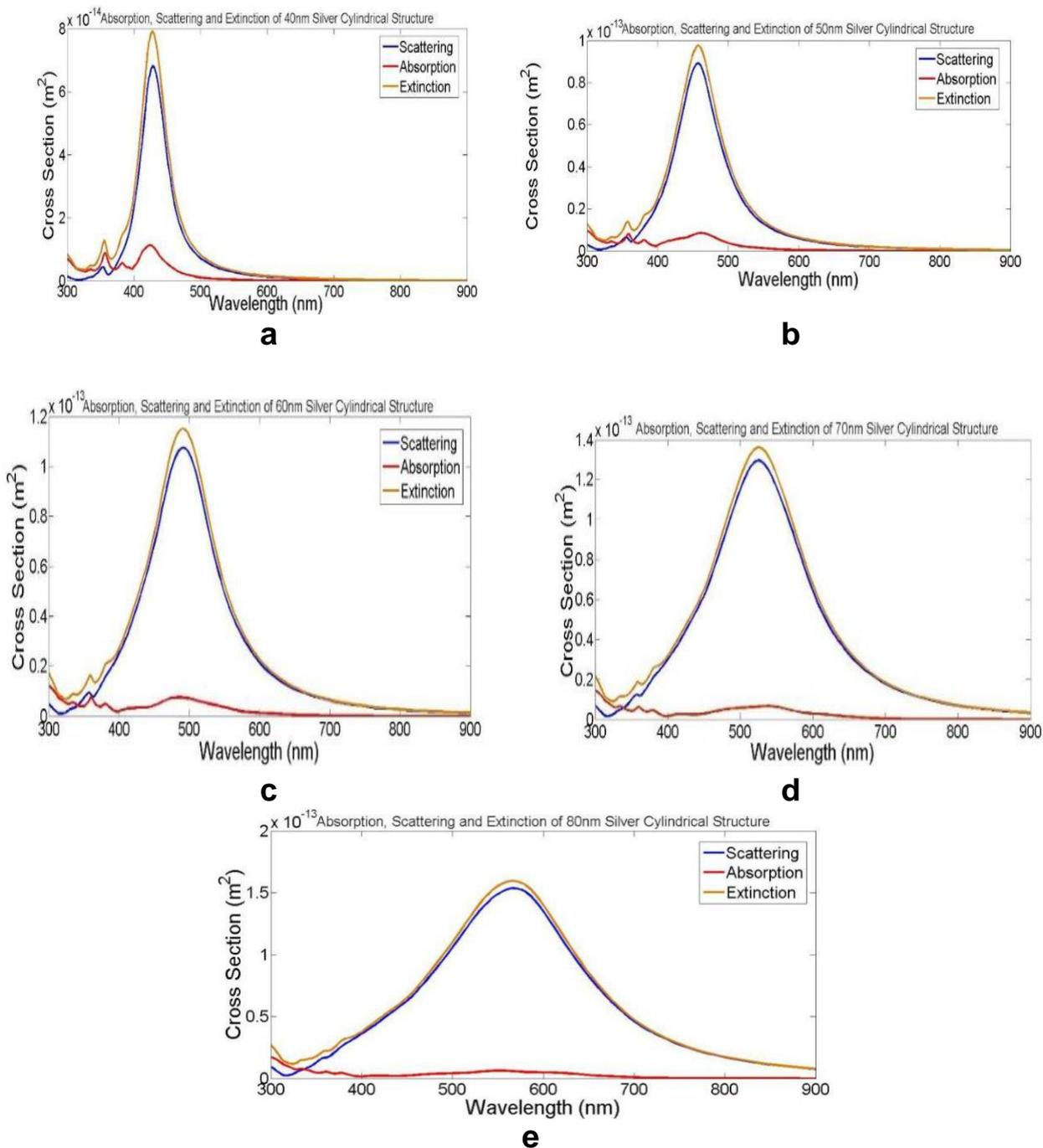
FIGURE 7: Absorption, Scattering and Extinction spectra for Cylindrical nanoparticle with 'r' a 40nm b 50nm c 60nm d 70nm e 80nm
