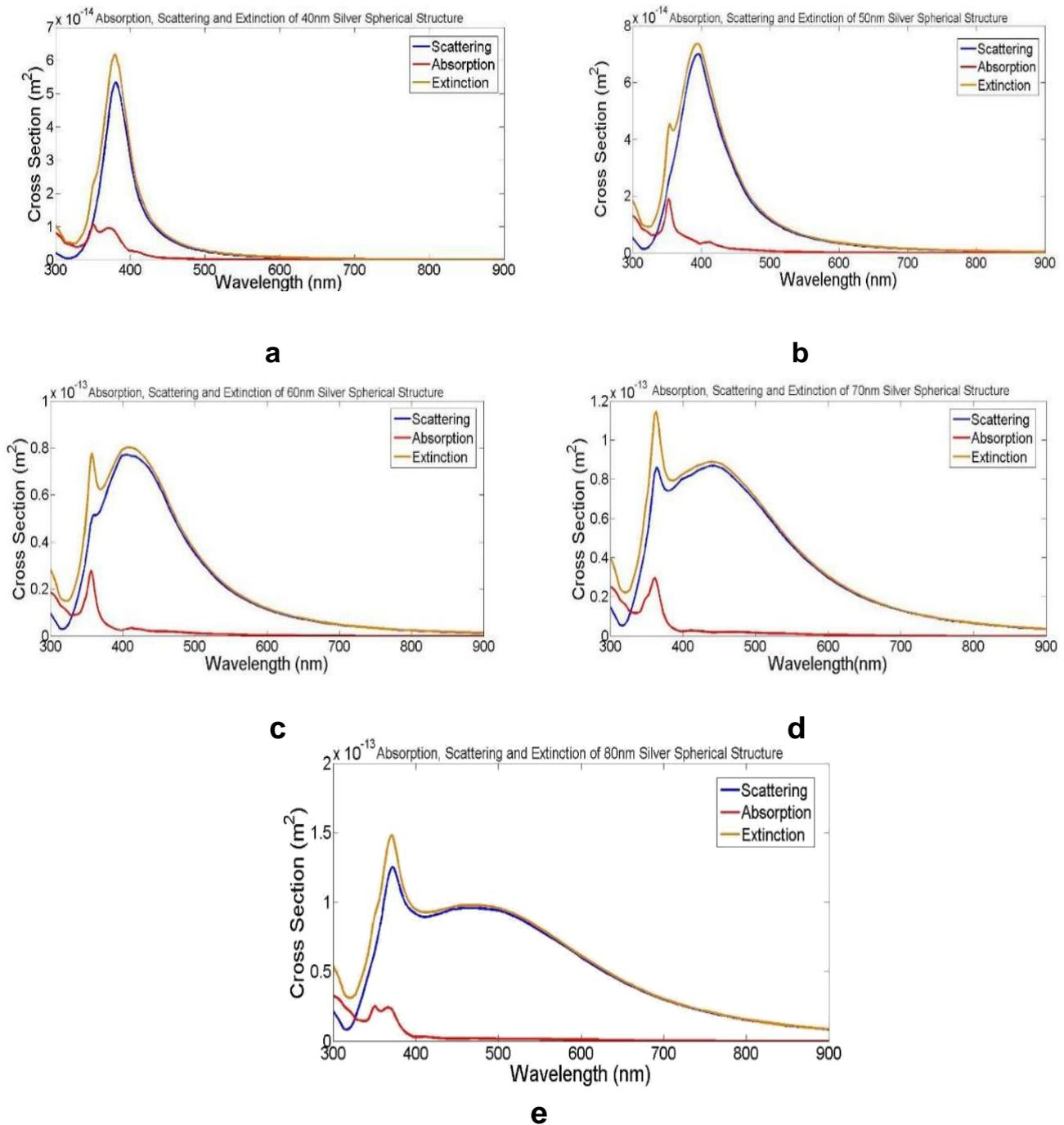
FIGURE 5: Absorption, Scattering and Extinction spectra for Spherical nanoparticle with 'r' a 40nm b 50nm c 60nm d 70nm e 80nm
