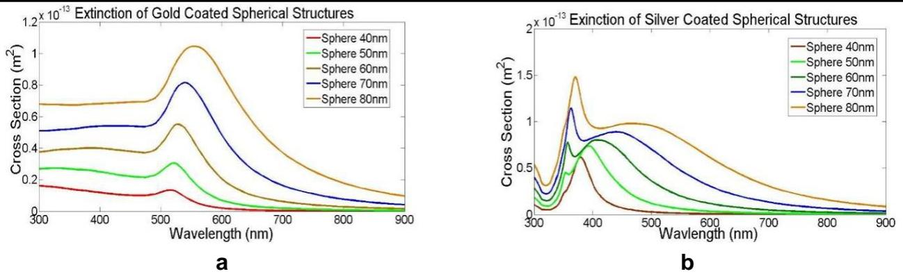
FIGURE 8: Extinction spectra for spherical nanoparticle a. Gold coated b. Silver coated
