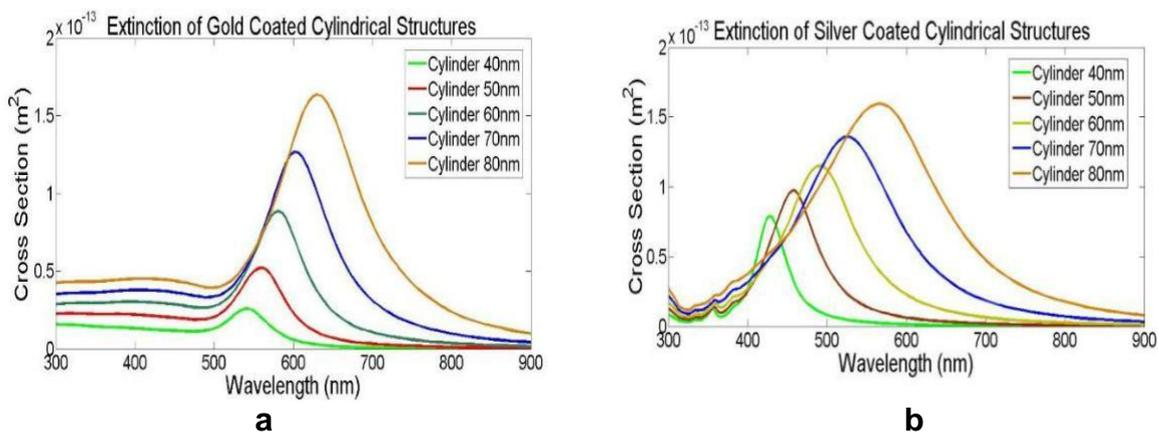
Fig. 10 Extinction spectra for Cylindrical nanoparticle a. Gold coated b. Silver coated
