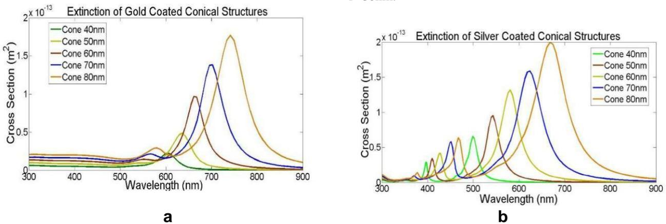
FIGURE 9: Extinction spectra for conical nanoparticle a. Gold coated b. Silver coated
