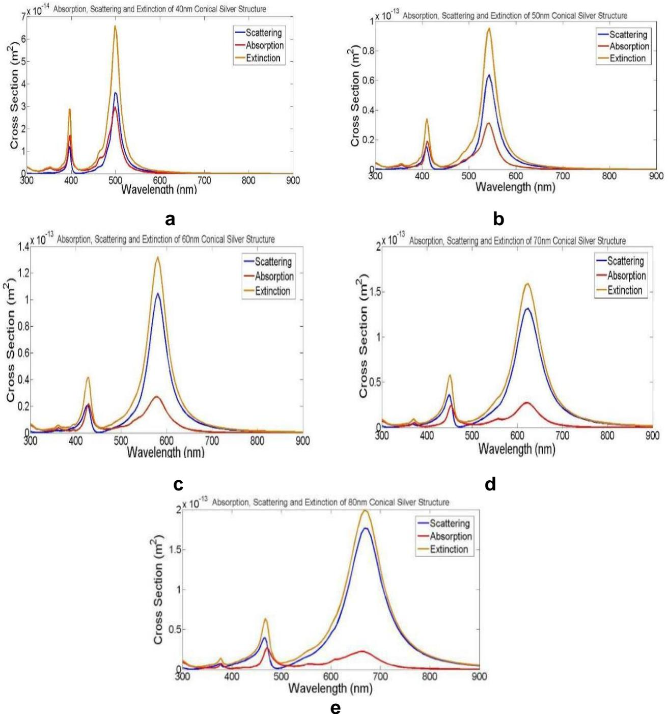
FIGURE 6: Absorption, Scattering and Extinction spectra for Conical nanoparticle with 'r' a 40nm b 50nm c 60nm d 70nm e 80nm
