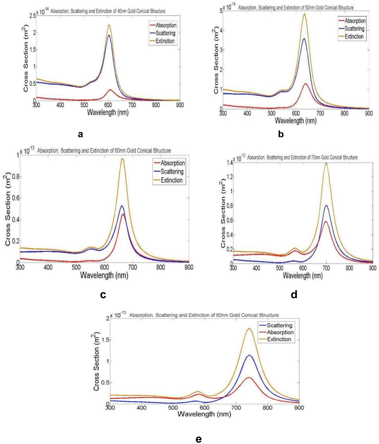
FIGURE 3: Absorption. Scattering and Extinction spectra for Conical nanoparticle with 'r' a 40nm b 50nm c 60nm d 70nm e 80nm
