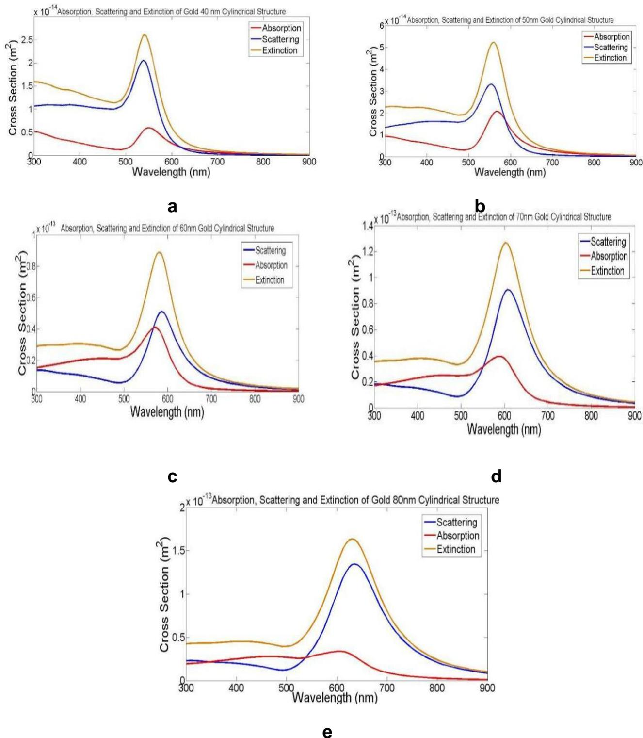
FIGURE 4: Absorption, Scattering and Extinction spectra for Cylindrical nanoparticle with 'r' a 40nm b 50nm c 60nm d 70nm e 80nm
