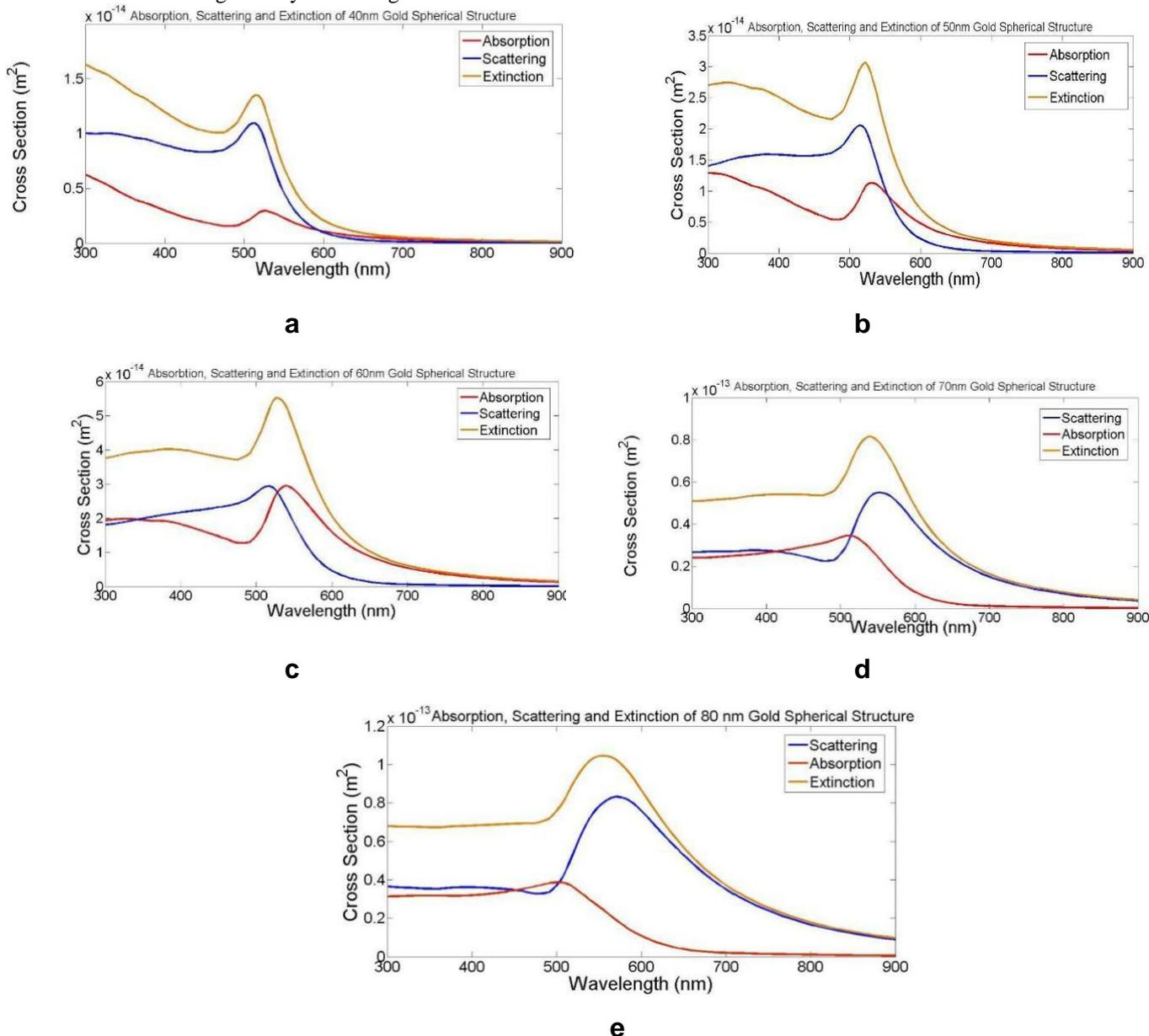
FIGURE 2: Absorption, Scattering and Extinction spectra for Spherical nanoparticle with 'r' a 40nm b 50nm c 60nm d 70nm e 80nm
